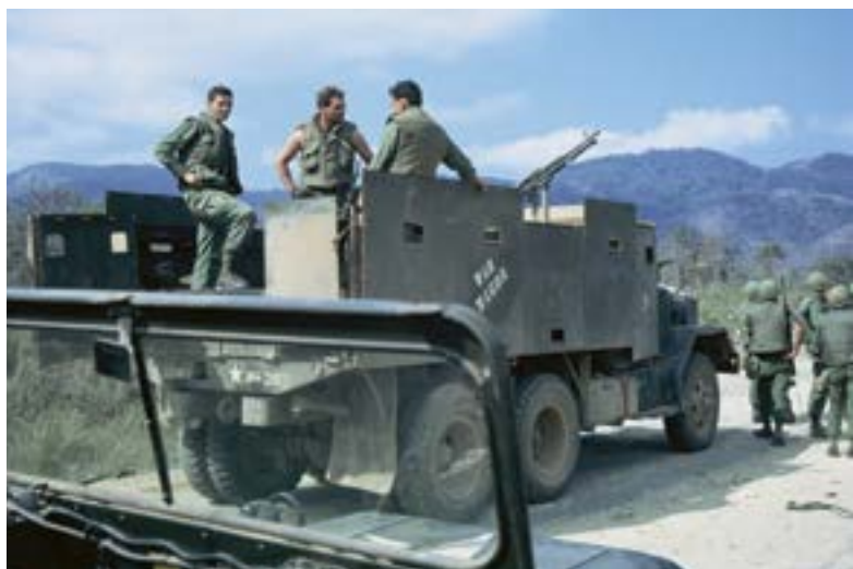
Typical design of 2½-ton gun trucks in the 359th Transportation Company with one plate shorter than the others. M-60s were mounted on pedestals.
