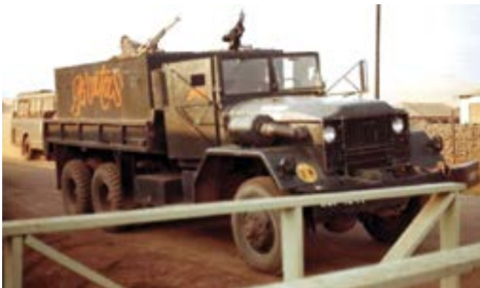
Brutus initially had twin .50s on back and later they were replaced with a .50 amd a M134 minigun.
