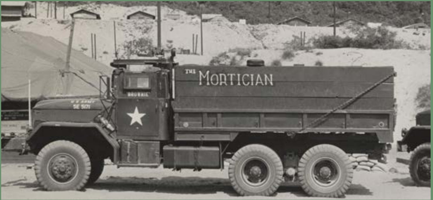
The Mortician. The first design of the guntruck in 500th Transportation Group were construction of either 2 X 8 or 2 X 10 inch wood walls reinforced with two layers of sandbags. Photo courtesy of James Bambenk
