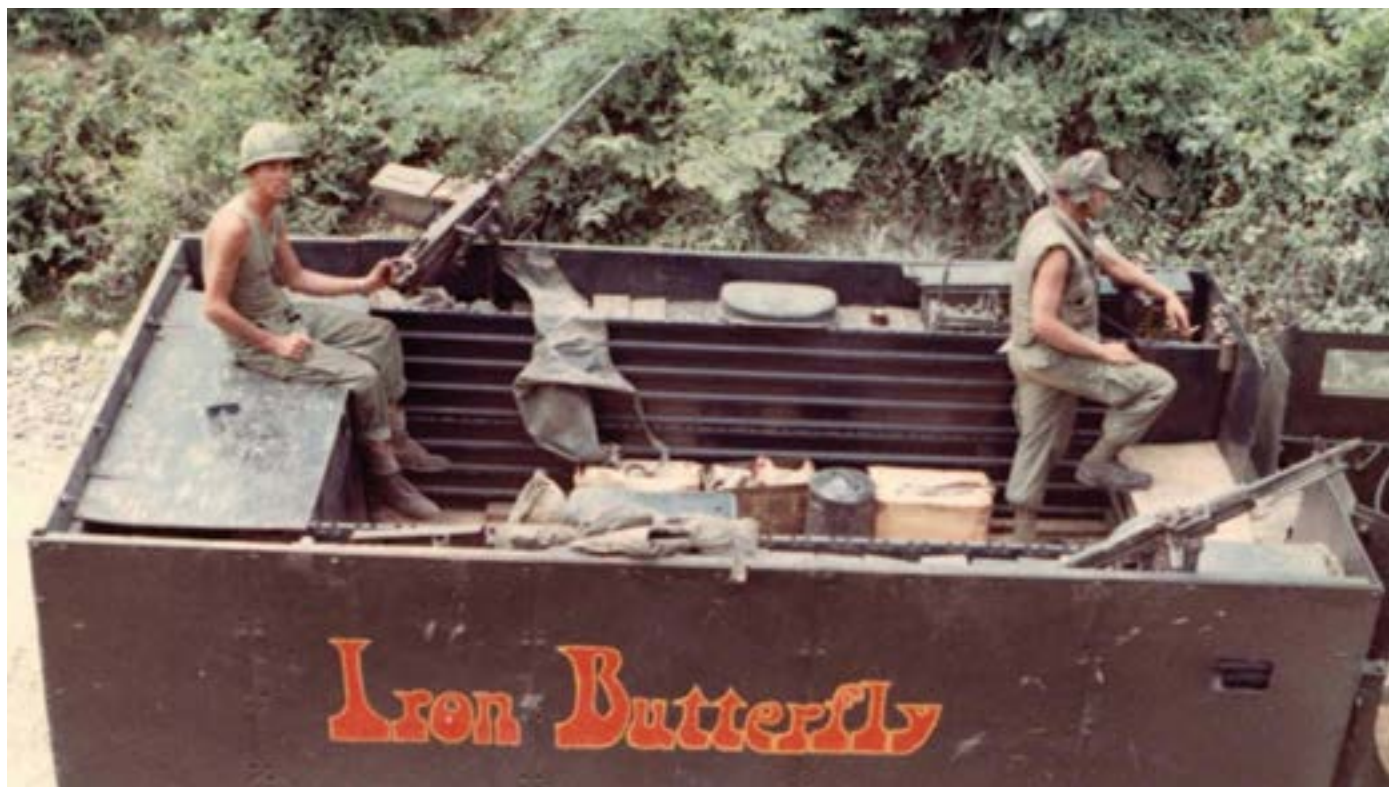
Iron Butterfly with two rear side mounted .50s and two forward side mounted M-60 machine guns.
