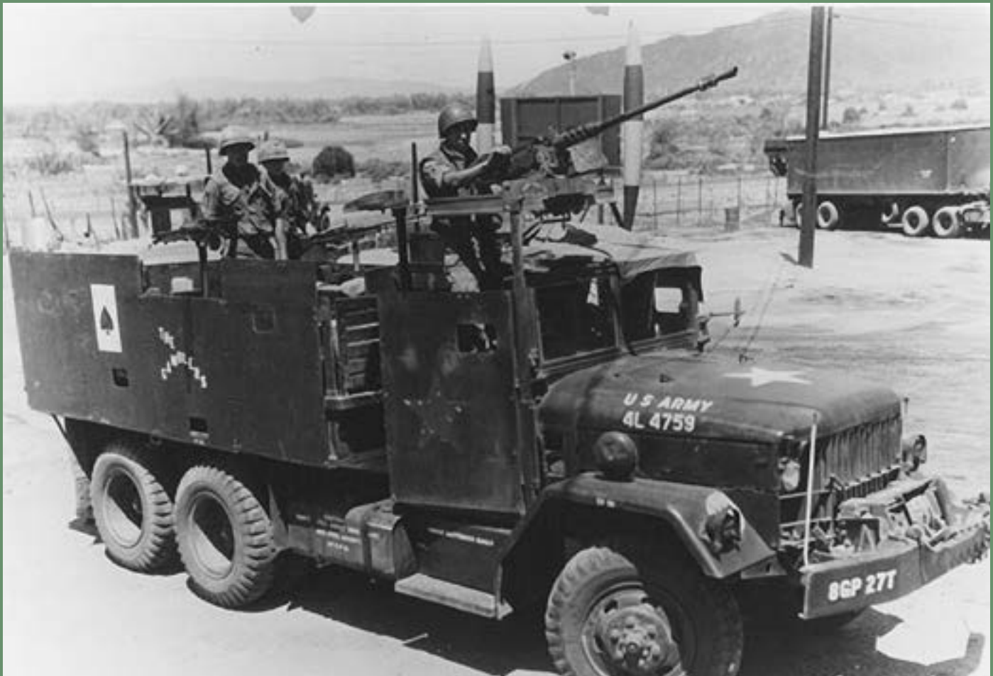
Gambler - Typical 8th Group 2½-ton gun truck with armored plating. This vehicle had sandbagged floors, 2 pedestal-mounted M-60 machine guns with sandbagged emplacements for added protection, and a M-79 grenadier. The vehicle was controlled from ring-mounted .50 cal machine gun. Photos courtesy of the US Army Transportation Museum
