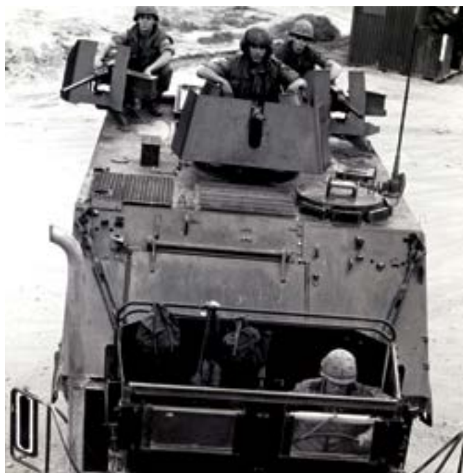
View showing gun and crew positions on King Cobra. Photo courtesy of the US Army Transportation Museum
