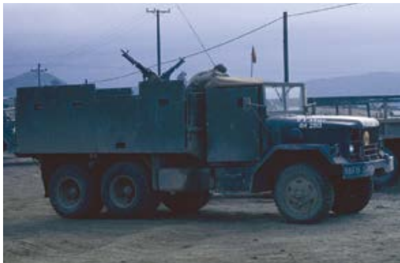
Typical design of 2½-ton gun trucks in the 359th Transportation Company with one plate shorter than the others. M-60s were mounted on pedestals.
