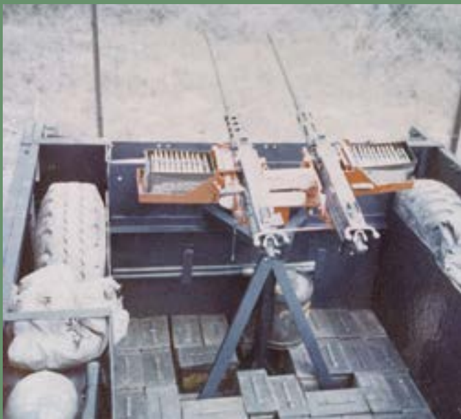
Rear view of gunbox of Eve of Destruction showing double wall and dual .50s. By this time, gun trucks carried as many ammo cans as would fill bed of the truck.
